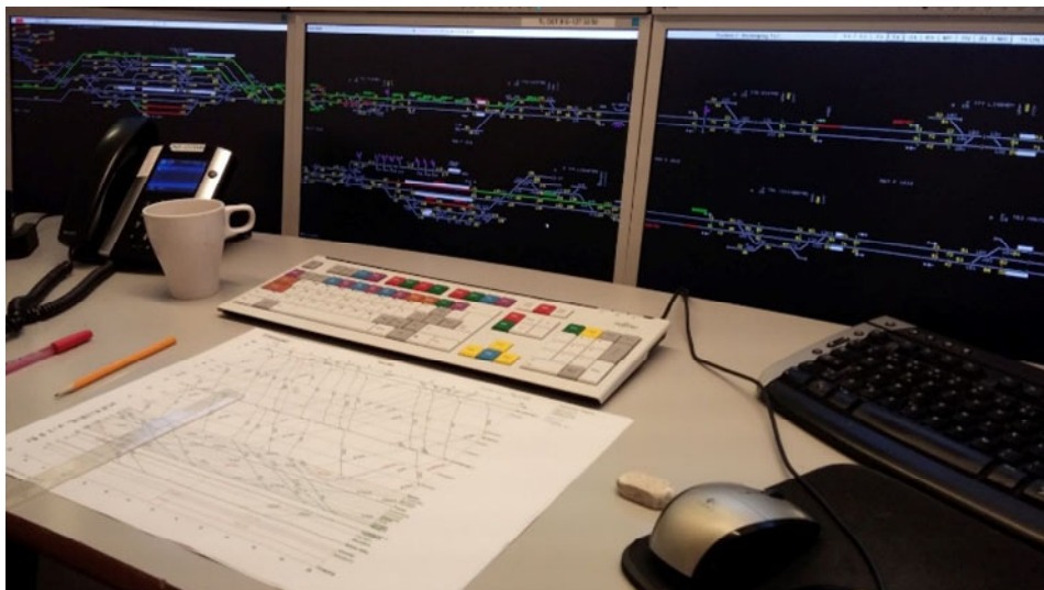
Figure 1 The workstation of a traffic controller includes the train traffic control system, the analogue paper-based time-distance graph and the telephone (see online version for colours)
