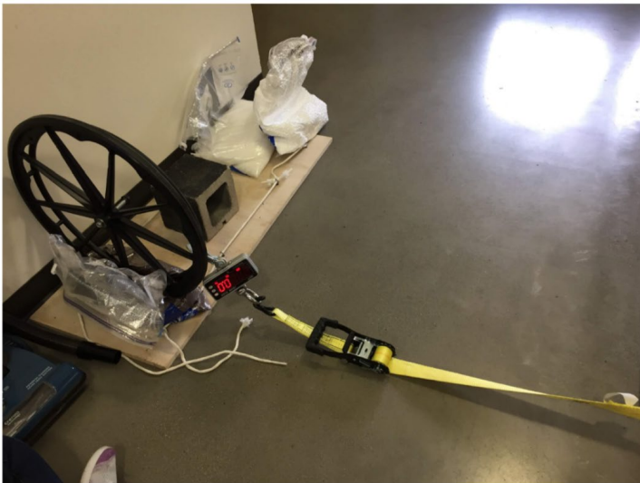
Figure F.23: Setup for testing the force required to pull the wheel of a wheelchair from particle jammed bags filled with different particles
