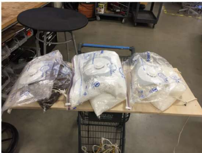
Figure F.22: Ziploc vacuum bags filled with (from left to right) coffee grounds, bean bag foam, plastic packing beads.
