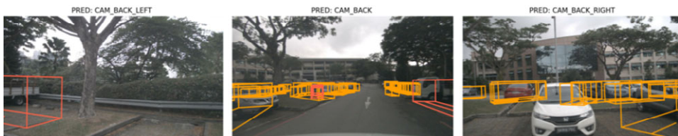
Figure 8 Visualisation of the MultiCAN-DEBEV model in a parking lot scenario with multiple vehicles and long-distance detection (see online version for colours)
